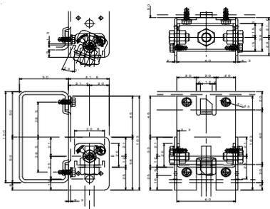
Fig. 3 Purlin reinforcement hanging bracket
