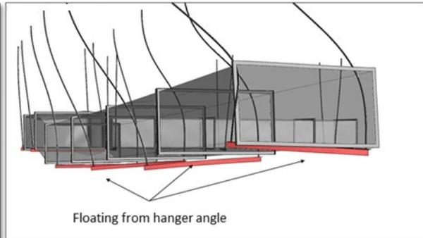
Fig. 7 Lifting from the hanger angle
