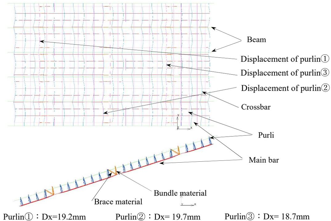
Fig. 6 Deformation status when horizontal acceleration is applied up to 3.67G
