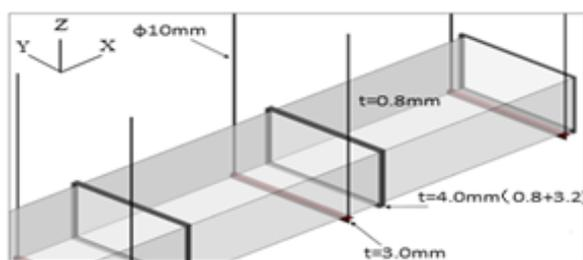
Fig. 5 Common plate flange clip fixing model
