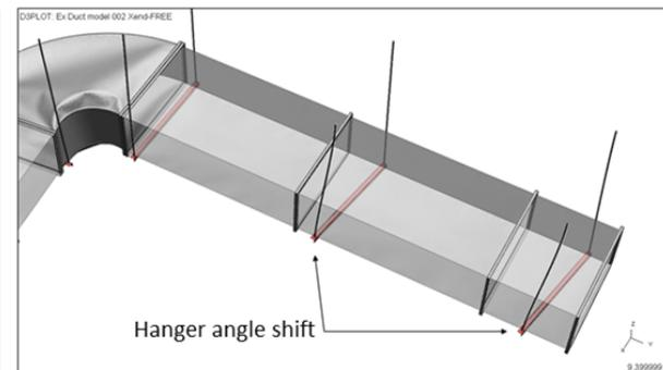
Fig. 9 Hanger angle misalignment
