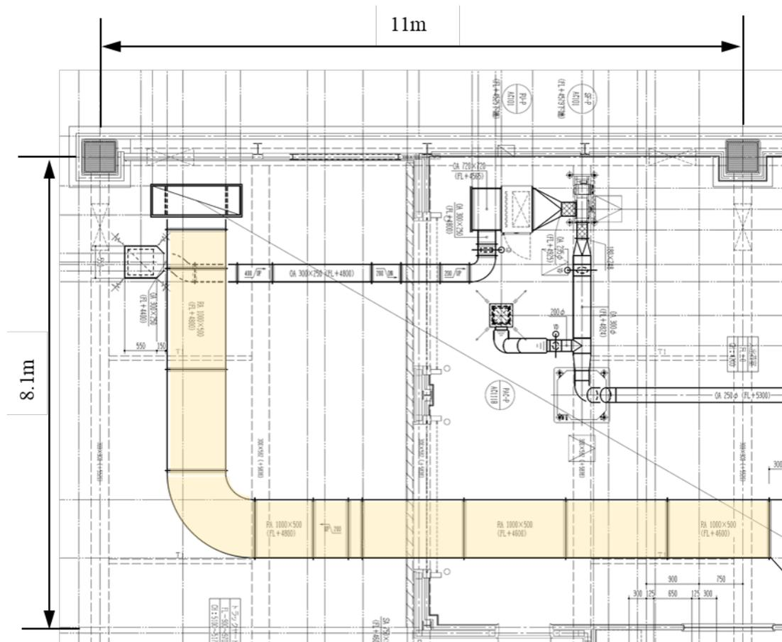
Fig. 2 Existing duct construction drawings
