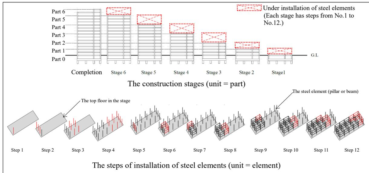
Fig.5 The stages and steps of installation of steel elements
