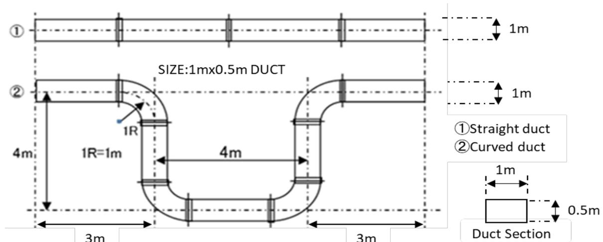
Fig. 1 Reference duct image diagram
