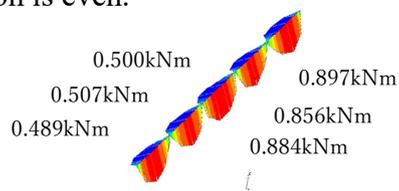
Fig.7 Bending moment distribution of purlin
