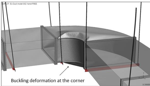
Fig. 8 Buckling deformation state of corners
