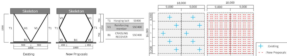
Figure 1 The model of the in-ceiling reinforcement
